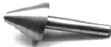
Another type of rotating center and known as a pipe center as it is intended for supporting work with large tapers.
