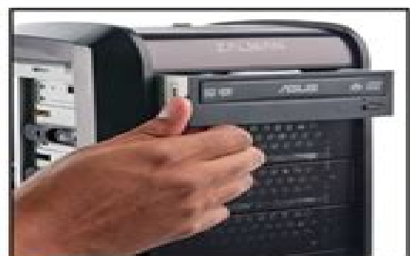
7 Install the optical drive
