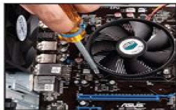
4 Mount the CPU cooler
