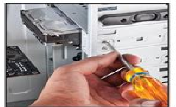
6 Install the hard drive
