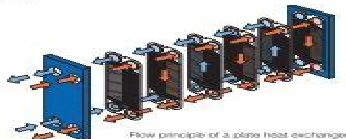
Flow principle of a plate heat exchanger
