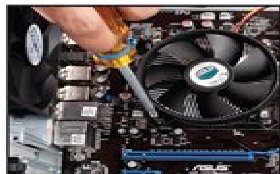
4 Mount the CPU cooler
