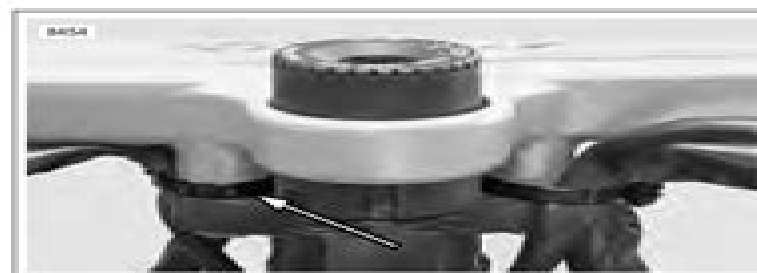
Figure 2-96. Cable Strap On Left Side of Upper Fork Clamp
