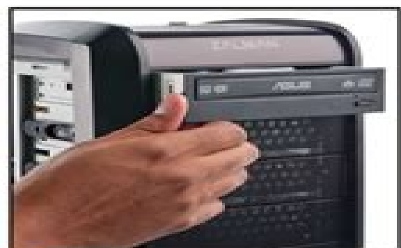
7 Install the optical drive
