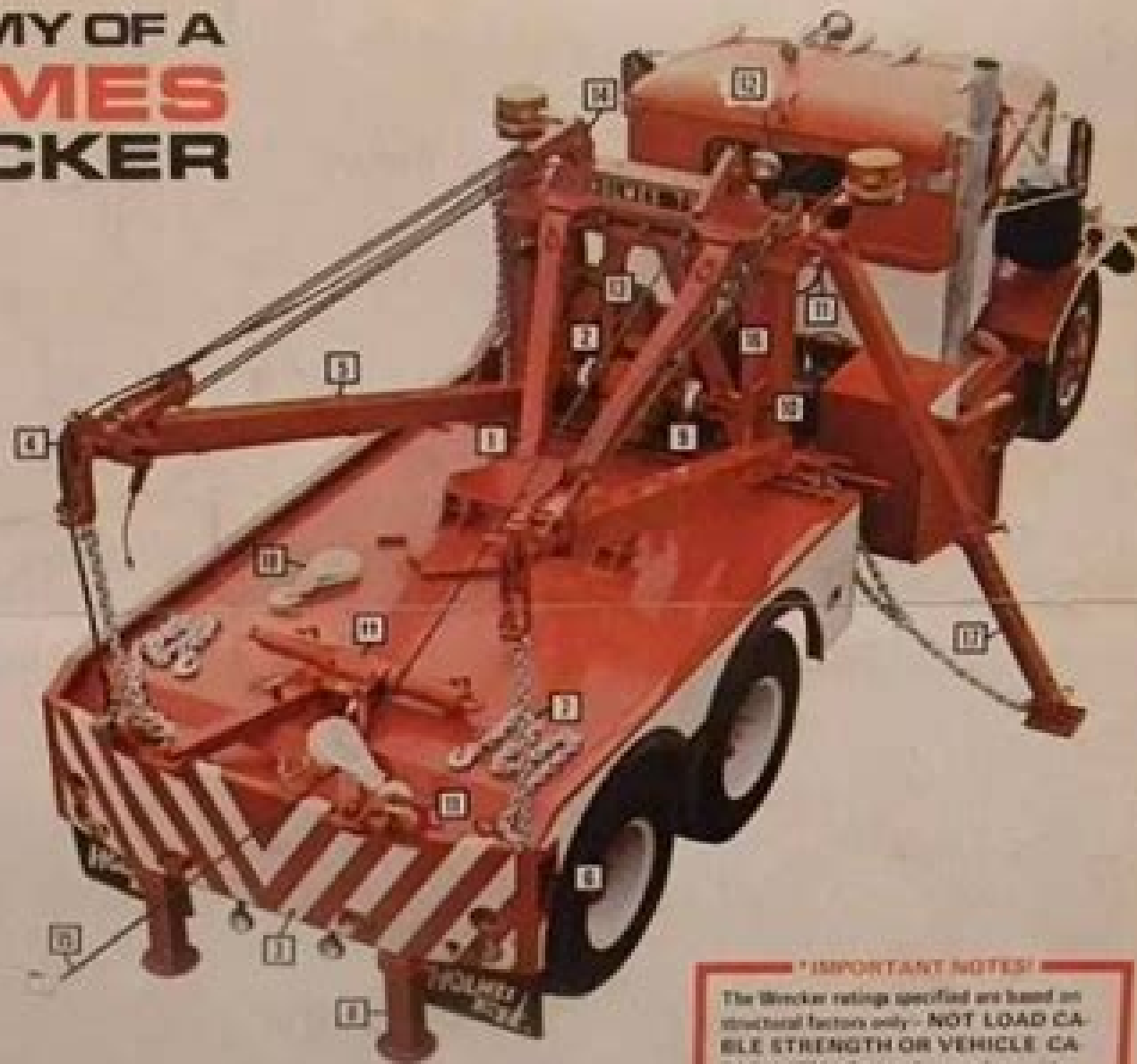
750" wrecker with extendible booms, Deluxe Heavy Duty Body and Truckmount Towing Hook.
