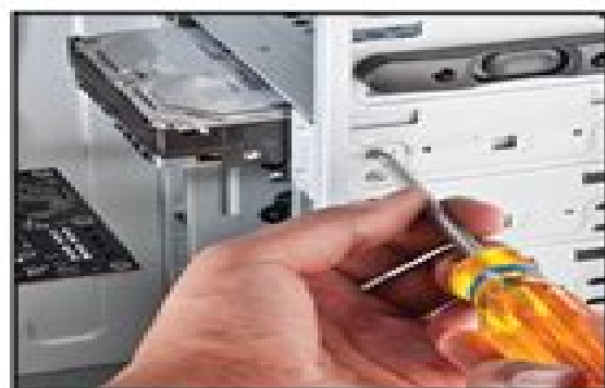
6 Install the hard drive
