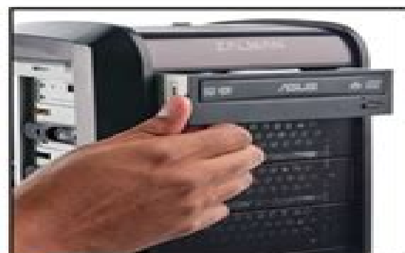
7 Install the optical drive
