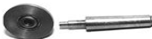
The parts of a homemade pipe center, showing the ball race that allows the head to rotate.
