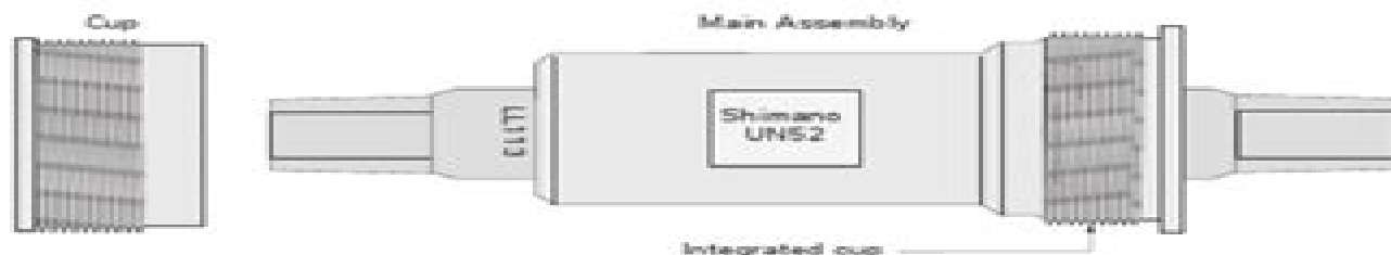
10.1 A typical two-part cartridge-bearing bottom bracket, consisting of a cup and a main assembly. There is a three-part variety which has a main assembly and two separate cups.
