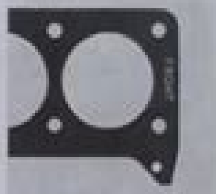
Fig. 47. Cylinder head gasket. The gasket should be seated in the guide.
