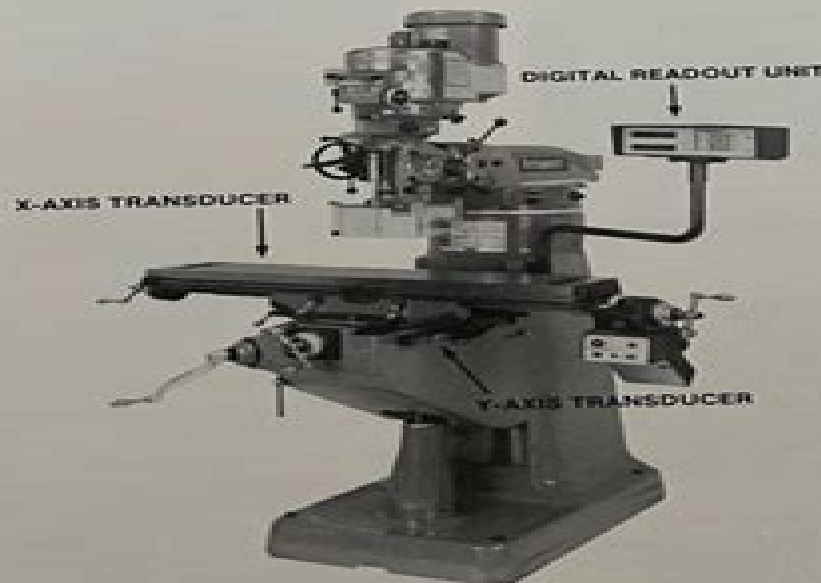
Figure 1-1: DRO System Components
