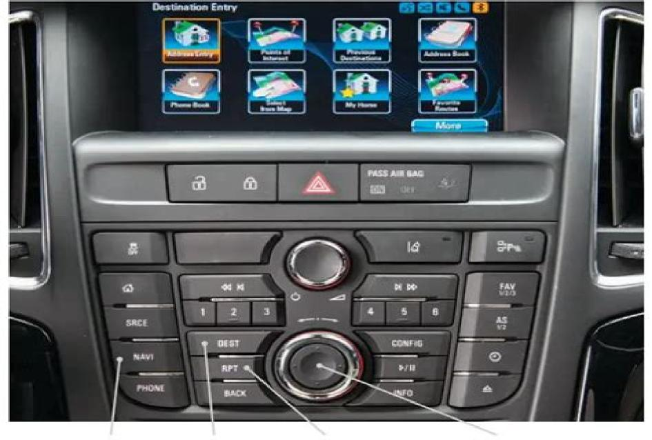
NAVI Map screens DEST Destination menus RPT Repeat voice guidance 4-Way Control: Move the 4-way control in the knob in different directions to move the map display
