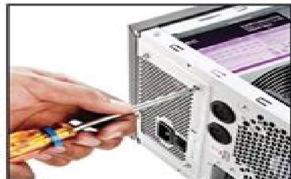
1 Install the power supply
