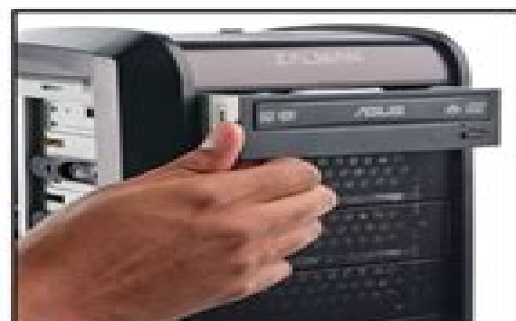
7 Install the optical drive
